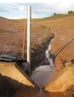
V nodge and limnigraph with data logger
